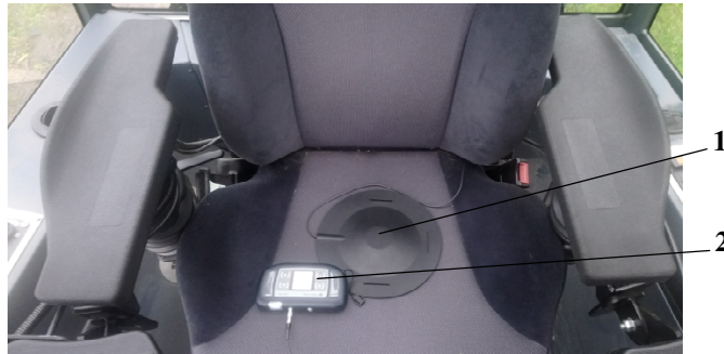
Fig. 3. Whole body vibration measurement instrumentation: 1 – seat pad accelerometer; 2 – human vibration analyser Bruel&Kjaer type 4447
