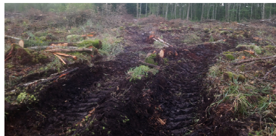
Fig. 3. View of the test site and the skid trail after multiple forwarder passes
